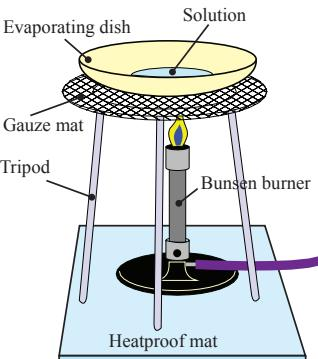
The diagram shows a laboratory setup for evaporation. An evaporating dish containing a blue liquid (labeled 'Solution') sits on a circular gauze mat. This mat is held in place by a metal tripod stand, which also supports a vertical glass tube. At the bottom of this tube is a Bunsen burner with a visible flame. The entire apparatus is placed on a light blue rectangular mat labeled 'Heatproof mat'.
